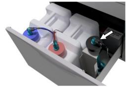
The process agent hoses only need to be placed head-first in the suction lance bracket if the metering hoses are to be bled, see Removing air from the metering system [ Page 23].
